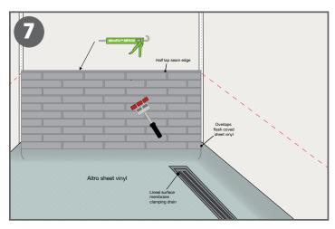
7. Install panel into proper position with correct spacing and aligned on or with datum line. Use a 3-wheeled wall roller to roll entire panel to ensure proper bond to wall substrate. Apply 1/16"(2mm) bead of AltroFix<sup>TM</sup> MP600 to the half-lap seam edge. Be sure to keep it above the visible seam edge.
