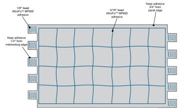
for cutting around penetrations, abutments and overall length of panel(s). Cut panels, and a best practice is always dry fit the panels and make adjustments if necessary before applying adhesive to the back of the panels. Leave a 1/16" (2mm) gap around the perimeter and around all cut-outs to allow for the expansion of panels.
