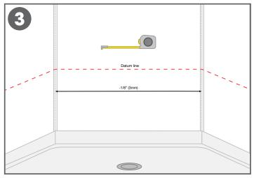
Measure the inside corner(s), cut the strips of A839 to length, and adhere them using AltroFix™ MP600.
