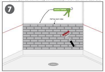
mix thoroughly. Apply adhesive to back of panel and/or to the wall substrate. Apply a bead of AltroFix $^{TM}$  MP600 to the internal corner of the previously installed A839 trims.
