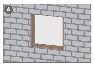
Install the panel per the Altro Tegulis installation guide. Be sure to use a wall roller over entire panel to ensure a proper adhesive bond to the substrate.
