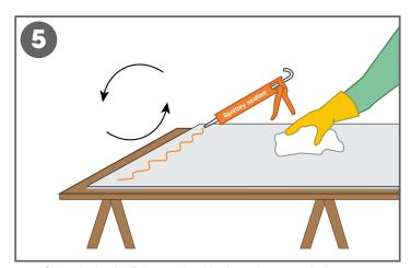
Clean the back of the panels with glass cleaner or similar to remove dust and contaminates. Apply Altro sanitary sealant on the back of the panel where it will overlap the existing flash coved flooring.
