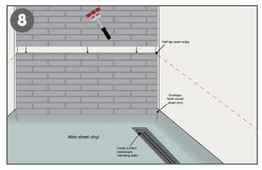
Install the top panel as previously instructed with correct space and properly aligned with the previously installed bottom panel. Use a 3-wheeled wall roller to roll entire panel to ensure proper bond to wall substrate.
