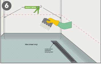
Depending on the environmental conditions and substrate, mixing of two-part adhesives may be necessary. Follow adhesive label and mix thoroughly. Apply adhesive to back of panel and/or to the wall substrate. Apply a bead of AltroFix™ MP600 to the internal corner of the previously installed A839 trims.
