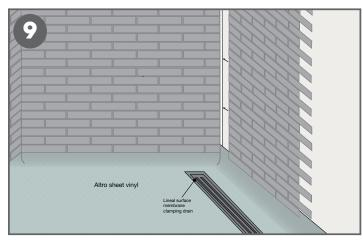
Additional wall panels that are not in direct contact with continuous moisture can be installed vertically with the interlocking joining method. This allows full panels to be installed without any horizontal seams. Install adjacent panels as previously instructed.
