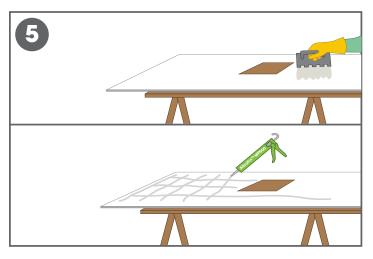
Apply Altro W39 adhesive with appropriate trowel or apply AltroFix<sup>™</sup> MP600 in a grid pattern.
