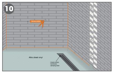
10. Apply Altro sanitary sealant as shown in drawing at inside corners, as well as top and bottom of all panels to prevent moisture ingress.
