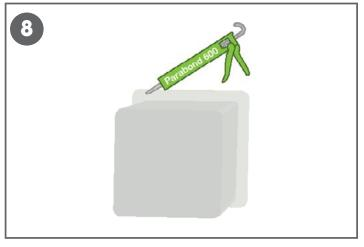
Apply AltroFix<sup>™</sup> MP600 to the back side of the flange. Install the recessed shelf and press/roll the flange area to ensure the adhesive bonds to the Altro Tegulis panel.
