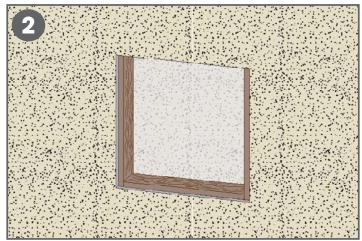
There must be adequate support within the wall substrate to hold the Altro Whiterock Recessed Shelf A900 and weight of its contents.
