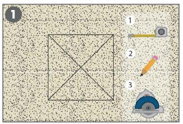
Use datum line or similar to determine location on wall substrate for placement of the Altro Whiterock Recessed Shelf A900. Measure, mark, and cut wall substrate accordingly.
