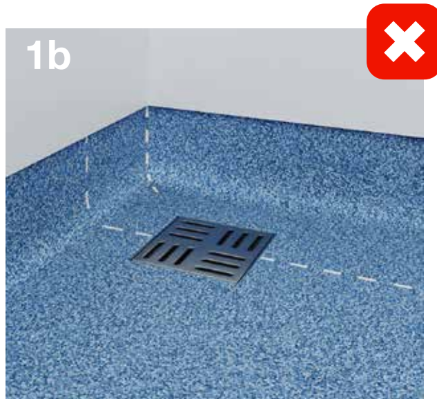
This shows the joint running across the drain.
