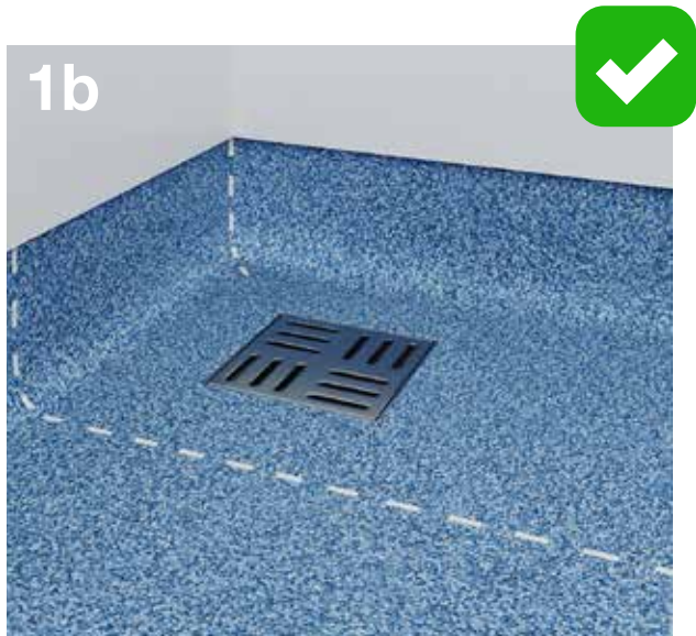
This shows the joint placed well away from the drain.
