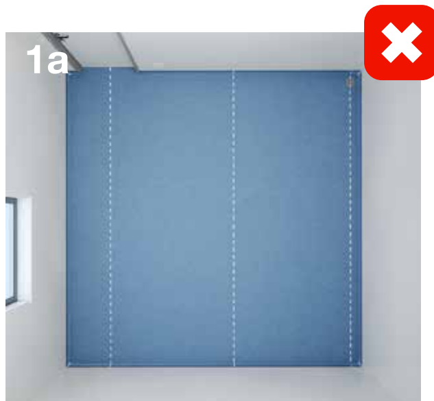
This shows the joint in the middle of the doorway (seen from above).
